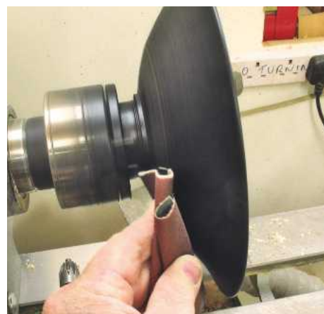
▲ Pic.18 Using coarse abrasive sand off the high parts of the texture. The more you sand the more colour you will get on the piece. Progress through the grits down to 400
